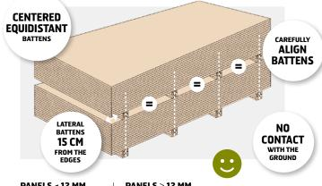
PANELS < 12 MM 250 x 122 cm: 4 BATTENS MINI 310 x 153 cm: 5 BATTENS MINI PANELS ≥ 12 MM 250 x 122 cm / 310 x 153 cm : 3 BATTENS MINI PLACE LOW THICKNESS PANELS ABOVE THE THICKER PANELS
