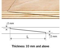
$$\label{eq:L} \begin{split} & \textbf{Thickness 10 mm and above} \\ & L = 8 \text{ times the thickness of the sheet,} \\ & \text{and maximum 170 mm.} \end{split}$$
